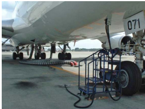
Fixed GPU (electricity / air conditioning)
